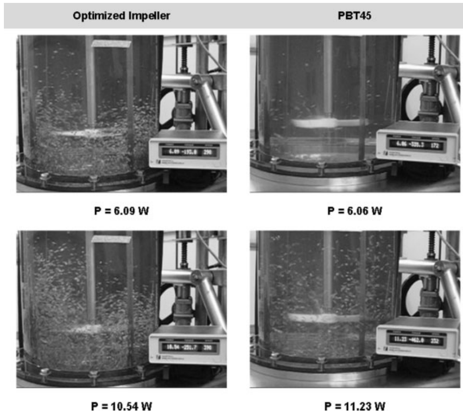
Figure 12. Experimental comparison between proposed impeller and the PBT impeller.
